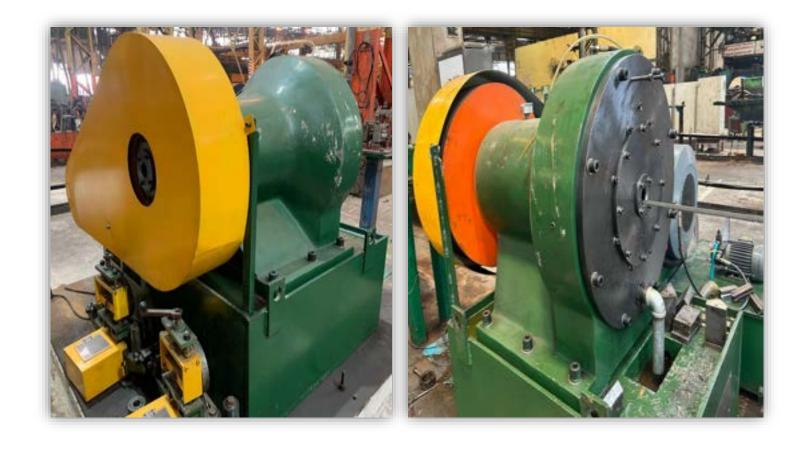
Swaging machines capable of diameter sizes upto ≤ 48 mm
